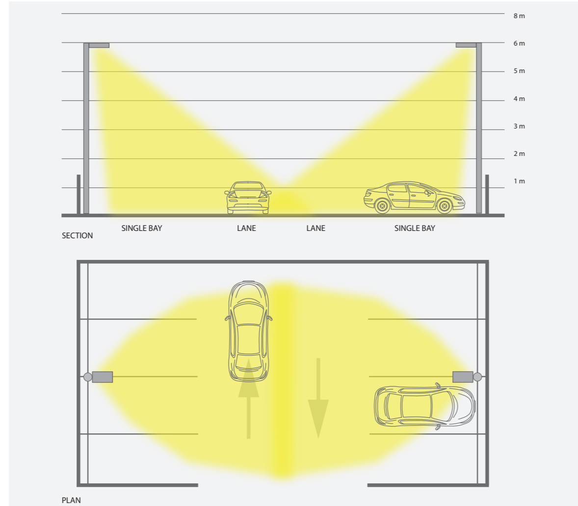
Single parking bay typical lighting arrangement
